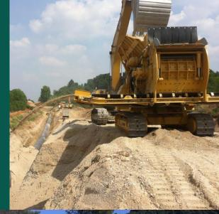
**HAMMER** offers the advantage of producing enough fine material to complete the protection of pipelines, even in rocky areas. The adjustable outlet grills allow for achieving the required grain size, adapting to project specifications.
