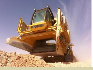
The **SUPERPADDER** is the largest model in Laurini's range of vibrating screens, with a **capacity** of up to **400** m³/h of fine material. With a **7** m² screening surface and a **3.6** m wide loading mouth, it's ideal for large projects. The remote control allows the operator to safely manage the input and output material from a safe distance, with perfect visibility.
